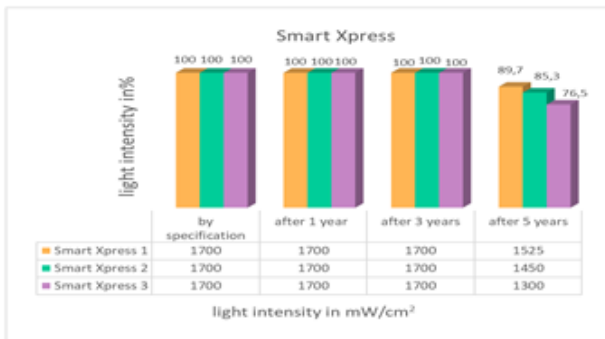
Fig. 12. Change in light intensity of LCU Smart Xpress (Bluedent) during 5 years period of use.
