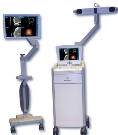
Fig. 3.** Neuronavigation device Medtronic® Stealthstation S7 using an infrared camera (localizer) and a reference frame with passive reflectors for navigation (BVM StealthStation 2021).
