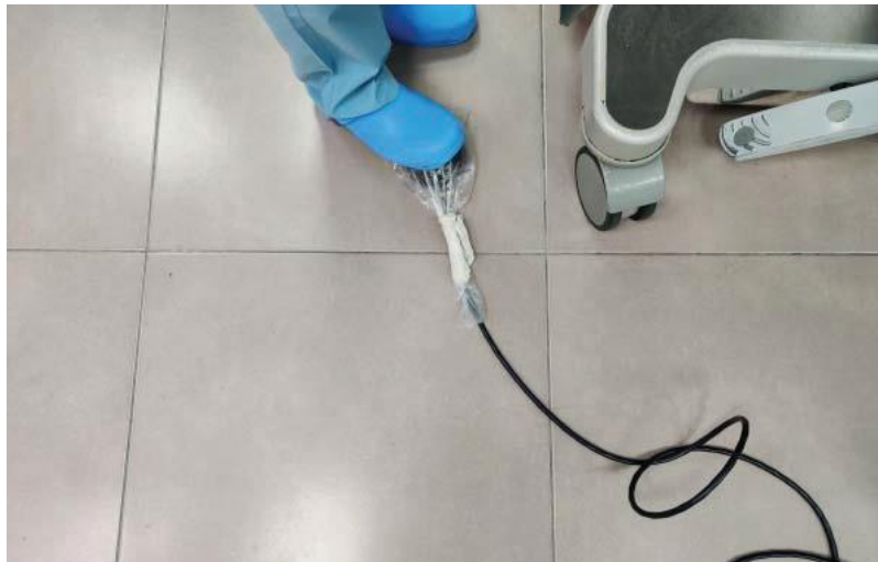
Fig. 32.* Working trajectory is locked by pressing the navigation pedal.
