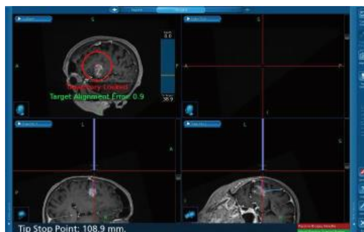
Fig. 33.* Locked working trajectory with deviation from planned target of 0.9 mm and marked biopsy needle length of 108.9 mm, at which the tip of the needle reaches the planned target point.
