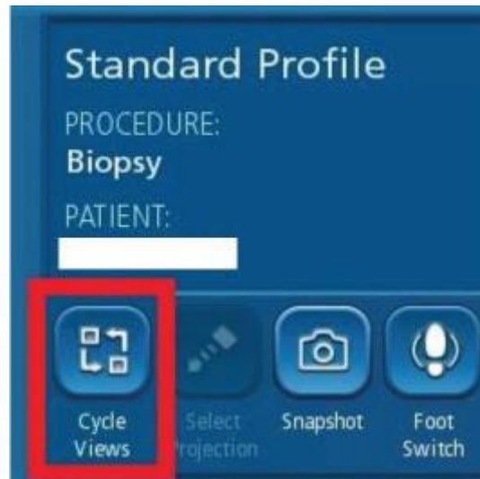
Fig. 52.** Mandatory screen refresh at each intervention in order to prevent the occurrence of an anomaly in the software related to the desynchronization of the depth gauge in relation to the rest of the navigation information (BVM StealthStation 2021)
