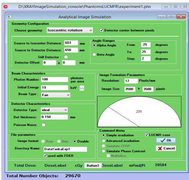
Figure 4.3. A view from the XRAYImagingSimulator for generating planar images in mammography and tomosynthesis
