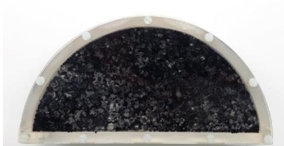
Figure 5.1. Picture of the physical breast phantom filled with water
