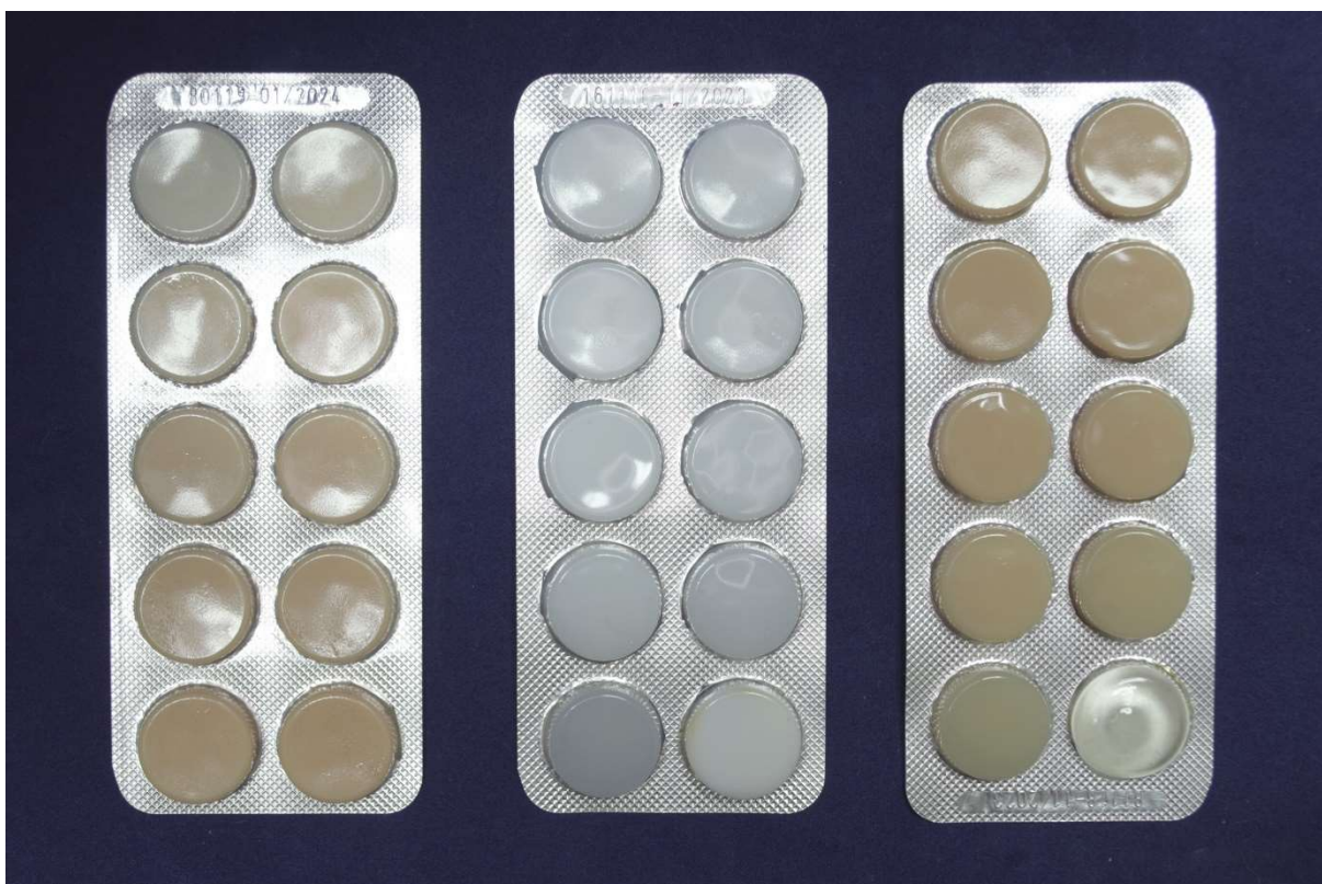
Fig. 16. Test samples after completion of the polymerization process.
