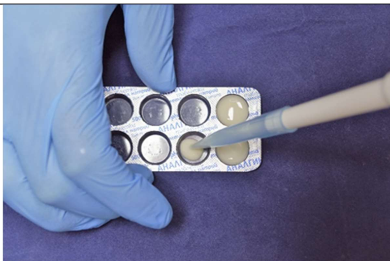
Fig. 14. Transfer of the composite resin to blister form.
