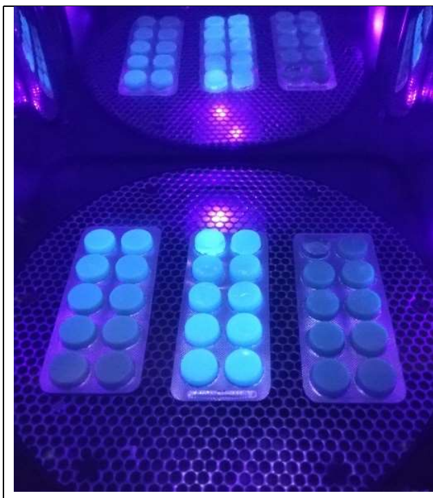
Fig. 15. Light polymerization of the test samples in the apparatus Form Cure®
