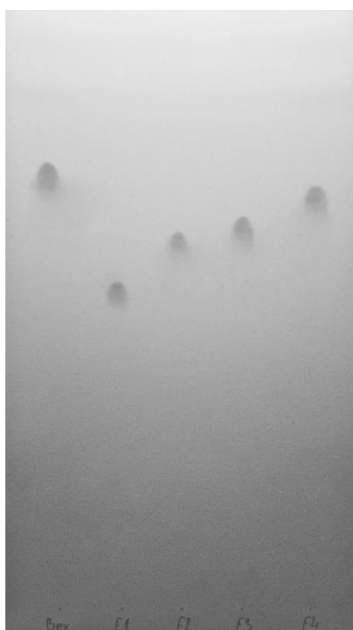
Figure 3. Thin-layer chromatographic analysis of Bexarotene and the newly synthesized esters E1, E2, E3 and E4.
