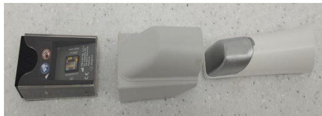
Fig. 21. Calibration Target for 3Shape Trios Intraoral Scanner
