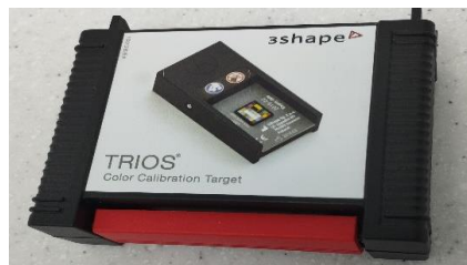
Fig. 21. Calibration Target for 3Shape Trios Intraoral Scanner
